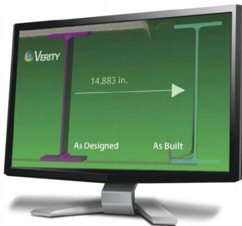
This process can be done by importing point cloud data into Navisworks and using a third-party plug-in application called Verity. Verity compares the point cloud data against the modelled data. It then provides feedback on what has been
